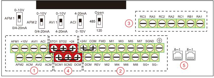
The control board is divided into 5 groups of terminals and connectors, plus a group of micro switches for individual terminal configurations.
